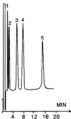
Fig. 4. Separation of mono- and bivalent ions. Chromatographic conditions as in Fig. 3; pH of the mobile phase, 4.2. Peaks: 1 = Na + ; 2 = Cs + ; 3 = Pb 2+ ; 4 = Mg 2+ ; 5 = Sr 2+ .
